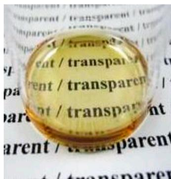
Fig. 1 Photograph of the phosphosilicate hybrid glass prepared from the (Ph<sub>2</sub>MeSiO)<sub>2</sub>PPhO oligomer.
