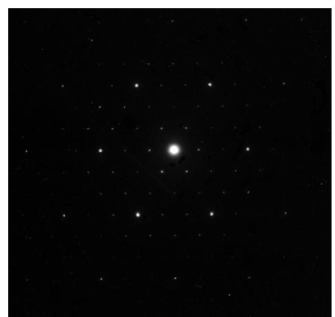
Fig.4 Electron diffraction pattern of P2VP single crystal at -197 degree.
